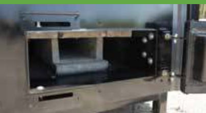
Secondary Combustion Chamber
