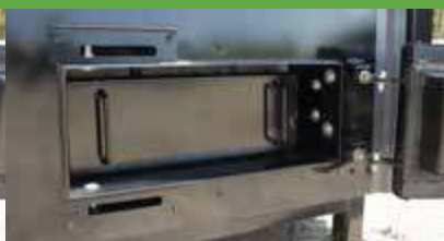
Secondary Combustion Chamber Heat Shield
